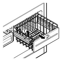
2. To Install, pull both rails out to full extension.
